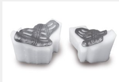
Additive Manufacturing Titanium Minimally invasive care for two orbital floor defects, including adjustment to partial anatomical models
